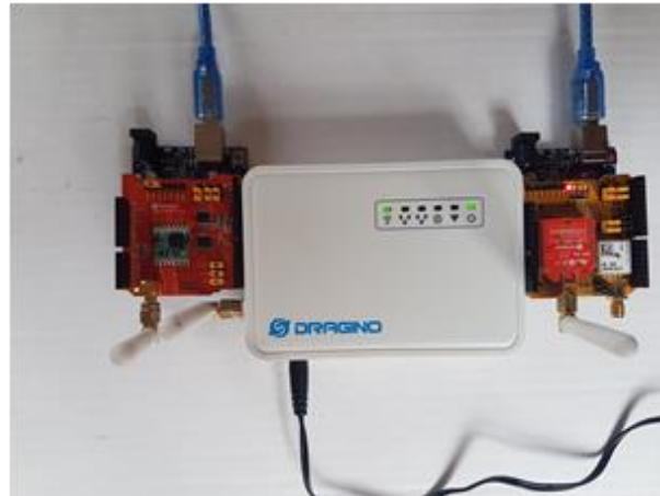
**Fig. 4.** Dragino LoRa gateway used for system
